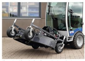
The cutting table can be tilt up for easy cleaning and maintenance. As an option, the mowers can be supplied with hydraulic tilting.
